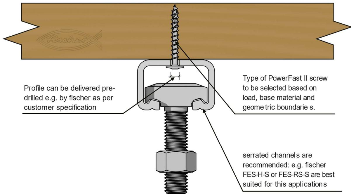
Figure G3.1: Applications of fischer PowerFast II screws with fischer FES-H or FES-RS-S (figure not to scale)
